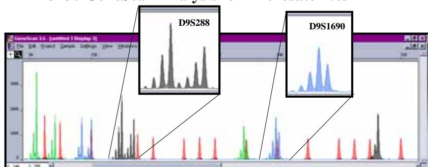
GeneScan Analysis plots (size (bp) vs. fluorescence intensity) of **microsatellites** on the 3100 Genetic Analyzer. GeneScan Installation Standard and the GeneScan 400-HD Size Standard run with POP4 and a 36cm capillary array are shown. The Installation Standard is a pool of six Linkage Mapping Set markers, amplified from an individual CEPH family member (1347-02).
