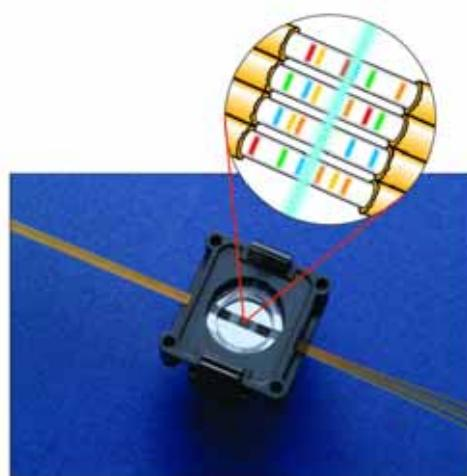
Close-up image of capillary array detection cell with a stylized schematic representation of in-capillary detection.
