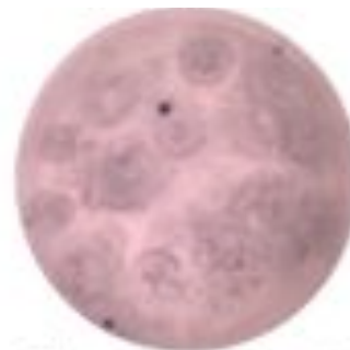
Plate was not thoroughly rinsed after developing and then dried flat:
