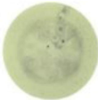
While pipetting, the pipet tip has touched the membrane
