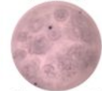
Plate was not thoroughly rinsed after developing and then dried flat:
