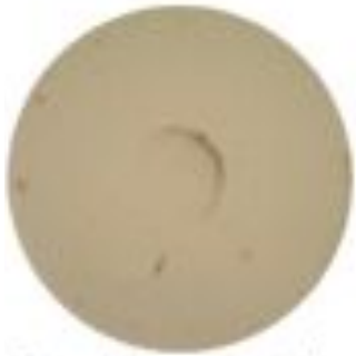
Pipet tip has pierced the membrane
