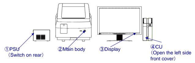
\*Switch on Main body before activating FV10i-SW
